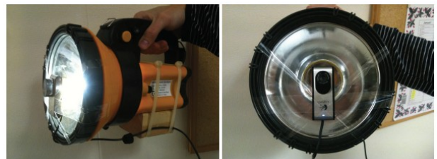
Figure 2. Experimental setup: rechargeable spotlight and a webcam glued to the center of its frontglass.
